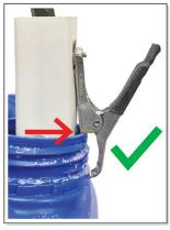
7. Add more water or remove some of the salt water to get the vent holes covered as shown in the picture.
