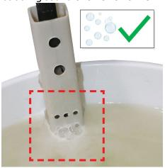
11. The unit will stop after the required time. Remove the bleach generator from the container. Rinse the bleach generator off with clean water.
